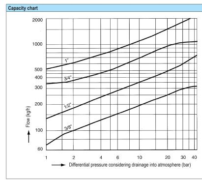
The capacity chart shows the maximum flow of hot condensate for the standard controller
