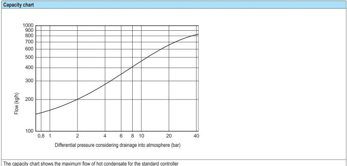
The capacity chart shows the maximum flow of hot condensate for the standard controller Flow rate of cold condensate at  $20^{\circ}\text{C}$  is about 1,5 times the volume of hot condensate
