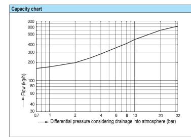
The capacity chart shows the maximum flow of hot condensate for the standard controller
