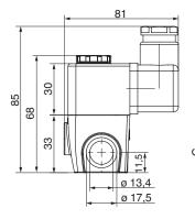
X: G 1/4 (connection code 14) G 1/8 (connection code 18) M5 (connection code M5)
