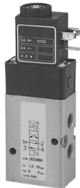
GEMÜ 8505 4/2-way metal pilot valve, servo assisted, aluminium DN 4 + 7 (1.0/1.5 - 10 bar)
