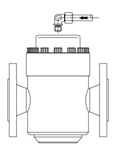
Operated by a smaller self-relieving pressure regulator. Reduced droop.
